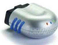
Hardware-based systems include the Progressive “Snapshot” dongle. The hardware device plugs into the vehicle diagnostic port and keeps track of mileage, and how often the driver slams the brakes. Verizon Telematics also has a hardware-based system called In-Drive for driving data, vehicle diagnostics, incident alerts, roadside assistance and stolen vehicle location.
